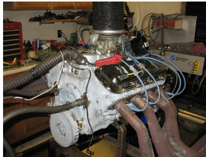
427 engine-now around 460 cu.in., on the dyno. 545 hp & 545 ft.lbs. of torque- Hang on tight!
