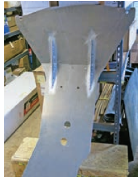
A large aluminum skid plate was fabricated to protect the bottom of the car, including the front cross member, transmission, and drive shaft.
