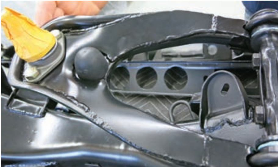
The front cross member was reinforced through some ingenious welding patterns.
