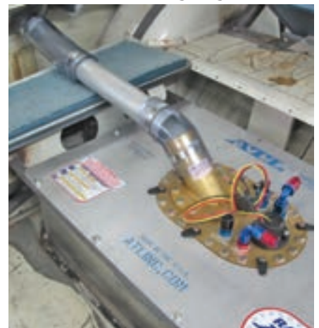
The fuel tank was replaced with an aluminum fuel cell holding 22 gallons.
