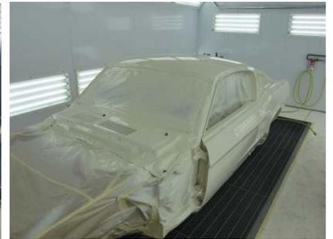
The Shelby GT 500 is now cloaked in a fresh coat of Glasurit single stage Wimbledon White paint. Our Paint Shop Manager, CJ Tremper, has taken great care to study the 100s of photos of this car and recreate the seam sealers, undercoatings, paint overspray, etc. to factory specs. We'll let the results speak for themselves.
